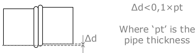
Figure 3 Acceptance criteria for misaligned pipes
